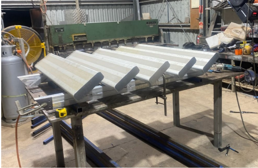
Figure 3: Fabrication of the container stairs
